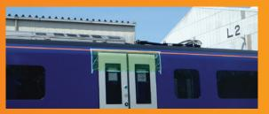
Running the length of all trains above door height is an orange line (shown in photo). Passengers should not raise anything above this height when exiting or boarding a train. It is a visual reminder to keep a safe distance from a train's overhead equipment.
